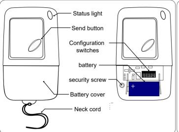
1. A battery is already installed in the Keyfob.
